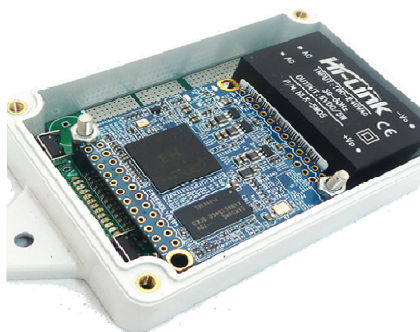
Fig. 4. Open-source device (openZmeter).
